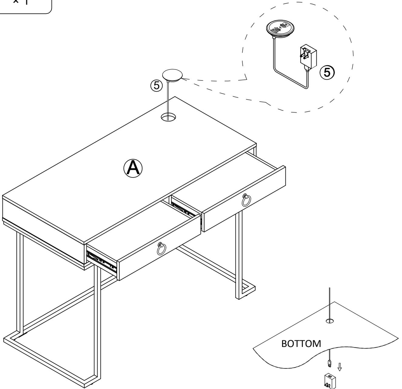
Note: Put the wire through bottom shelf hole firstly, then connect wire with plug.
